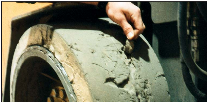
Deteriorated joints can cause extensive damage to material handling vehicles, resulting in reduced operational productivity and excessive MHV maintenance and repair costs.
